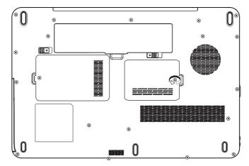
Figure 8-5 Seating the memory module cover
